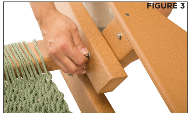
Step 5. Using a 4" button head bolt in upper hole, secure left outside upright. FIGURE 4
